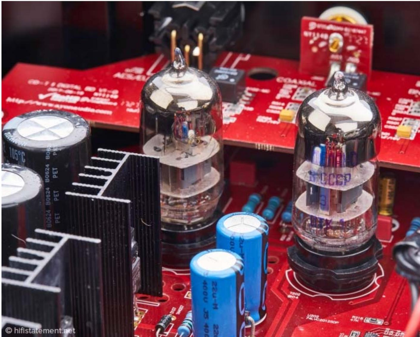
*Oops! Did the tubes accrete? The previous model got along with one double triode. The solution: the second tube only works for the digital BNC output and will only be implemented with the PCM-DSD board.*
