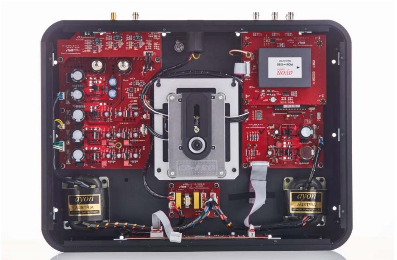
*At the first glance the inner design resembles the old machine, disregarding the additional DSD module. However, e.g. the power supply has been redesigned completely.*
