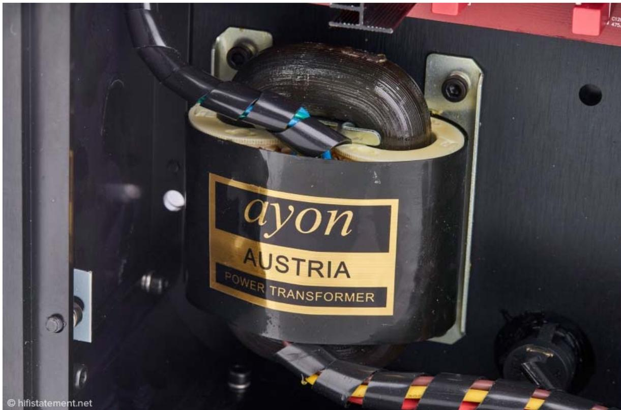
*Remained are the highly efficient and R-core transformers of low dispersion, especially produced for Ayon. The device contains two transformers for the separate supply of drive and signal. In general, the power supply has been improved, what should be noticeable in a better playback of impulses.*
